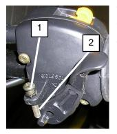
To limit throttle travel and top speed, the ATV is equipped with a throttle adjuster screw. The screw can be turned in to lower the top speed and out to increase the top speed. After adjustment, the locknut must be tightened down against the throttle housing.
