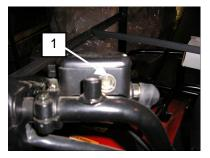
NOTE: When checking brake fluid, the ATV must be on level ground and the handlebars must be straight. If fluid level is low add DOT 3 only.
